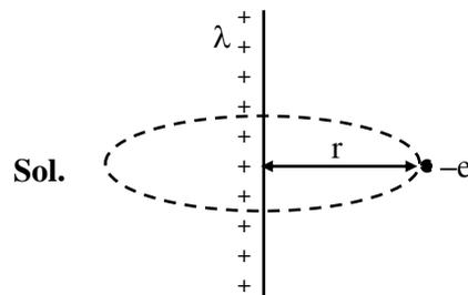
Electric field  $E$  at a distance  $r$  due to infinite long wire is  $E = \frac{2k\lambda}{r}$
