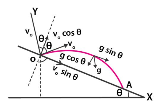
When x and y axes are selected as shown in the diagram, the motion of projectile from O to A is
