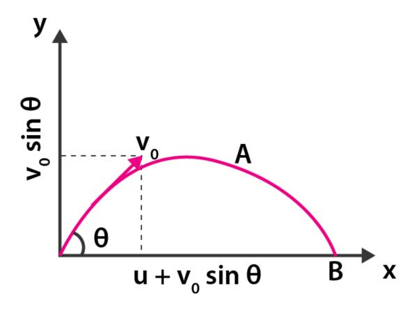
a) The angle of projection with the horizontal with respect to spectator is:  $\tan\theta=u_v/u_x$
