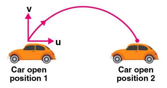
Above is the diagram which is viewed by the observer on the footpath. The diagram is parabolic as the vertical and horizontal components of the velocities are viewed by the observer.
