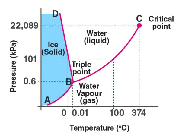
The above graph is between the pressure and the temperature for water. As the pressure increases, the ice changes into liquid state and when the pressure is decreased, it changes into liquid state.
