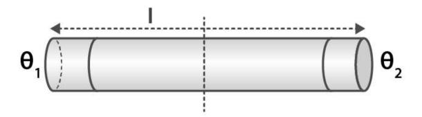
Above is the figure of a rod that has a uniform mass M and length l which is bisected perpendicularly.
