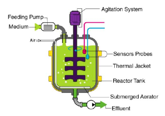
Flask is used for small laboratory scale testing of culture, and bioreactor is used for commercial-scale production.
